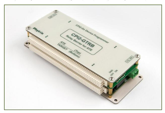
A CPI2-GTRB unit should be powered from an external 12 to 18V@2A power supply. The unit has a couple of two-pin green power connectors to plug a cable or wires from the power adapter, which can be connected to either side, wherever it is more convenient. These connectors are located on both short end faces of the CPI2-GTRB unit. See the CPI2-GTRB side view below.
