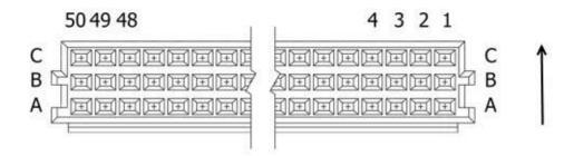
The matrix below shows pinouts of ISP and GND signals on the input male type connector located on a rear side of the relay barrier unit docking to the CPI2-Gx device programmer's **TARGET - channel A** and **TARGET - channel B** outputs.
