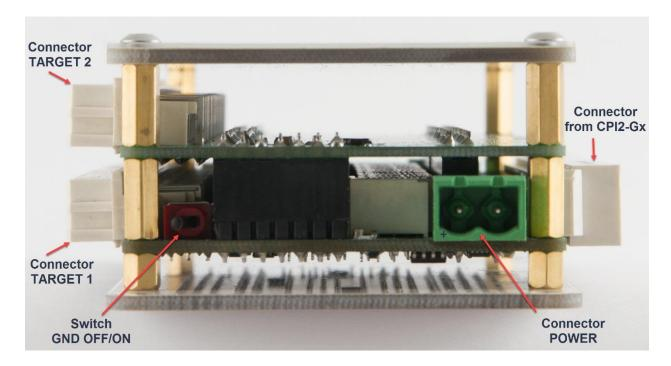
A CPI2-GTRB unit docks to female type **TARGET – channel A** or **TARGET – channel B** 150-pin DIN connectors installed on CPI2-Gx device programmers by a male type complimentary connector marked on the top label as **CPI2-Gx Device Programmer**. This connector locates on a long rear side of the CPI2-GTRB unit.
